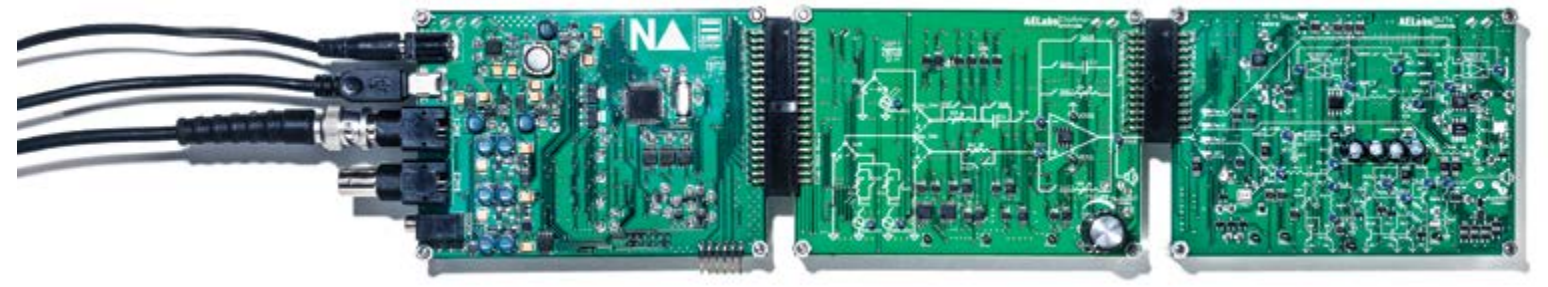
The NileDelta board interfaces electric power, user activity, and external stimuli which are then used to configure the analog circuits on the auxiliary AELabs boards.
