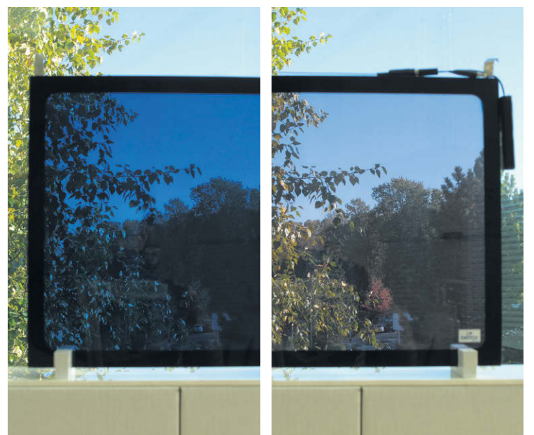
Technology developed by SWITCH Materials will allow drivers to control the tint of their windows with the flick of a switch. SUPPLIED
